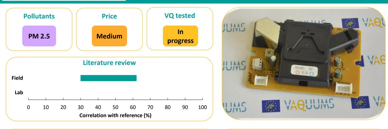
The Shinyei PPD60 detects air borne particles sized over 0.5  $\mu$ m based on the light scattering method. The air is self-aspirated by the air current generation mechanism with a built-in heater.
